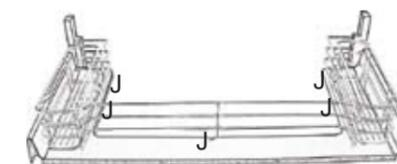
6. To secure the bin lid support to the end panel, four 5mm holes will need to be drilled into the end panel. The top-right hole should be drilled at 218mm (in) x 261mm (up - from the top of the bottom panel). Secure the bin lid support using 4 M screws.
