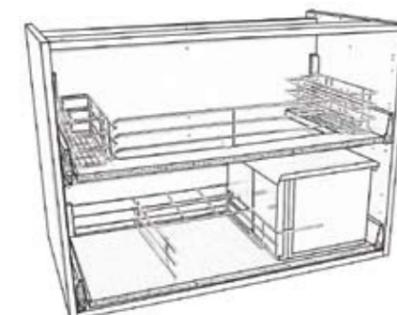
7. Fit the drawer runners into the 1000mm base unit, in positions 2\* and 5, using M screws. Once fitted insert both drawers.
