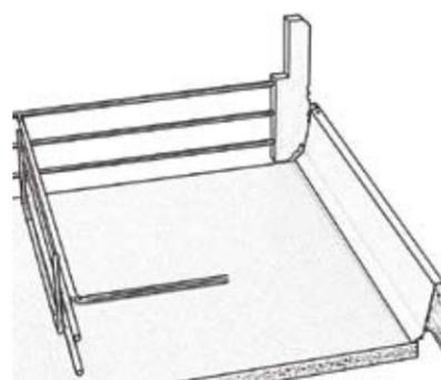
4. Fix the wirework divider in place where required. Secure the wirework, using 4 x J screws. Use these to keep the wirework square.
