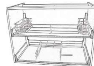
8. PLEASE NOTE: there is a Top and a Bottom drawer front. When attaching the drawer fronts, although this unit uses a 450mm depth drawer, please use the top holes on the drawer front to fix the gallery rails. Remember to lock the cams on the underside of the drawers when fitting the drawer fronts.
